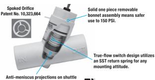
Anti-meniscus projections on shuttle prevents shuttle from drying in place after long machine shutdowns.
